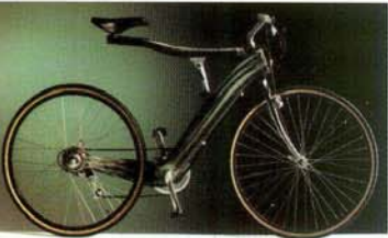
Lightweight construction using reinforced polymers: a monocoque bicycle frame.
