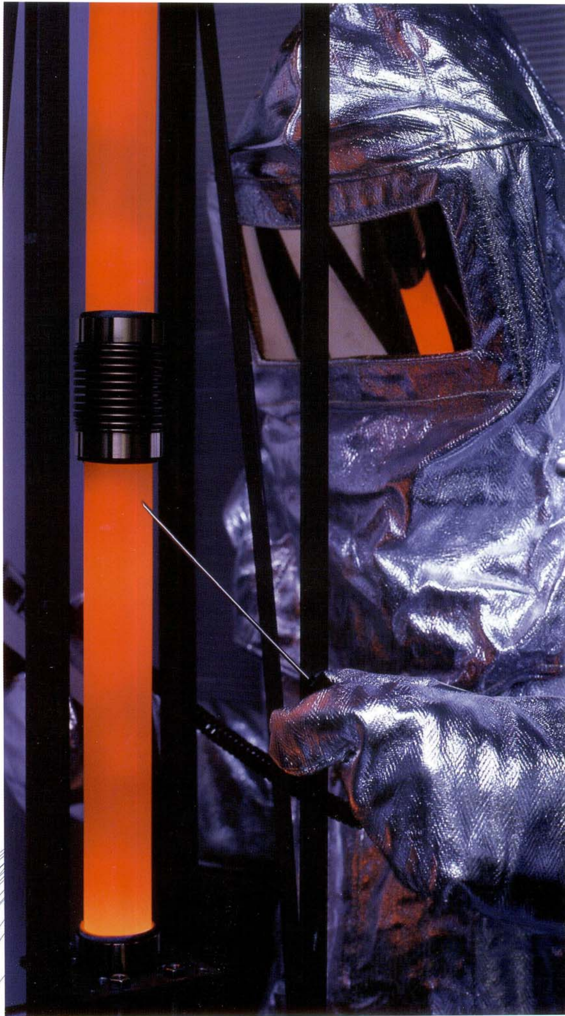
Diesel soot – no thanks! Electrically regenerating ceramic filter plugs in a pilot test. Photo: Peter Winandy
