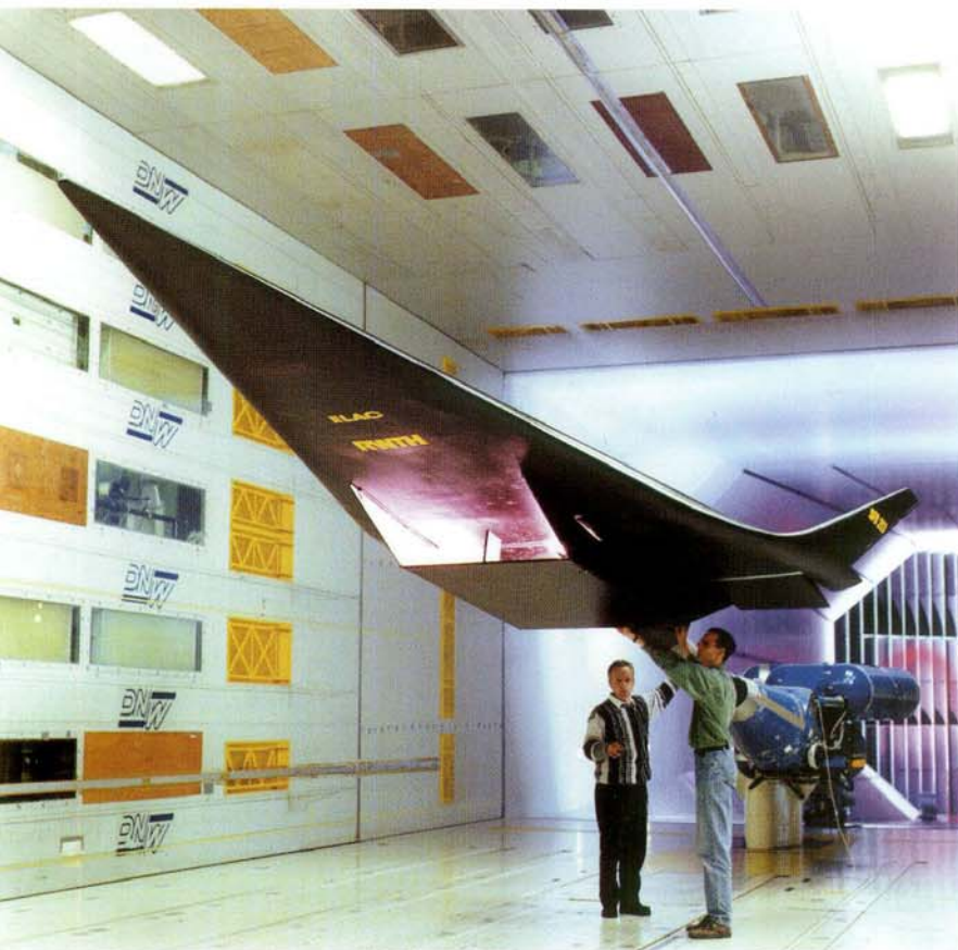
Spacecraft model in the German-Dutch wind tunnel DNW (model length: 6 m).
